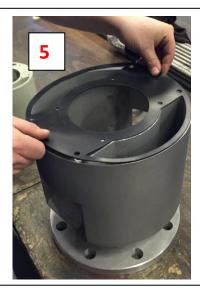
6. Place newly supplied Aluminium Ring on top of newly supplied NBR cover gasket. 7. Make sure it is the right way up! See picture 7. Please note that the chamfered side of the aluminium ring has to be on the bottom, so that the new cover gasket will seal off properly as ball sealing. 8\*. Fasten bolts of aluminium ring. Bolts are to be tightened with max Nm torque, see table below for more info. 9\*. Replace cover and fasten bolts. Bolts are to be tightened with max Nm torque, see table below\*
